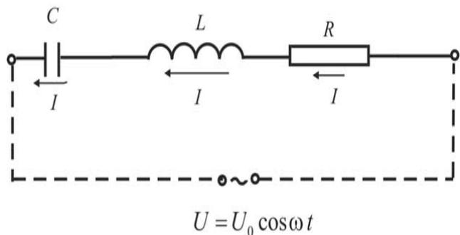
$$I = \frac{U}{Z} = \frac{U}{R + i\omega L - i\frac{1}{\omega C}} = \frac{U_0 e^{i\omega t}}{|Z| e^{i\phi}} = \frac{U_0 e^{i\omega t - i\phi}}{|Z|},$$
