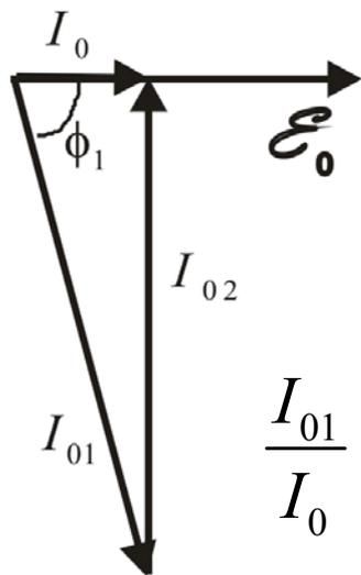
$$\text{tg} \phi \approx \frac{\omega^2 L^2}{R} \left( \omega c - \frac{1}{\omega L} \right) = 0, \text{ если } \omega^2 = \omega_0^2 = \frac{1}{Lc};$$
