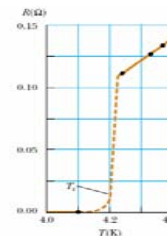
Figure 27.12 Resistance versus temperature for a sample of mercury (Hg). The graph follows that of a normal metal above the critical temperature T_c . The resistance drops to zero at T_c , which is 4.2 K for mercury.
